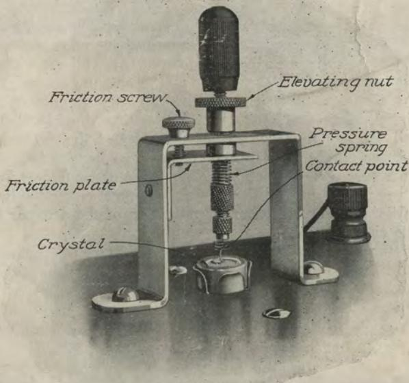
The elevation of this member can be varied by means of the milled elevating nut and the pressure spring serves to maintain the entire contact member at the elevation determined by the position of the elevating nut. The contact member is supplied with a ball joint to give
